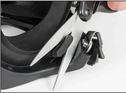
To mount a microphone into the mask, follow the manufacturer's recommended mounting instructions. In almost all cases, you will need to open up one of the communications ports, which are located below the bottom edge of the mask frame. Secure using tie wrap, KMDSI P/N 520-038.
