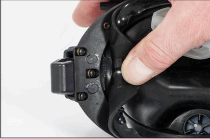
Over a period of time it might be necessary to increase the tension on the pod hook found on the left hand side of the pod due to material fatigue. If two clicks are not audible when connecting the pod to the mask, it is time to service the pod hook.
