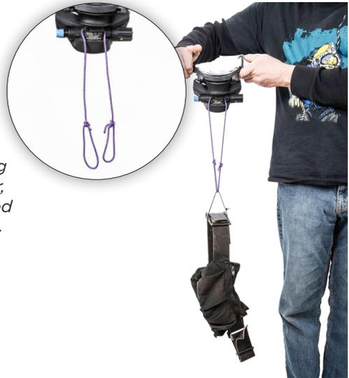
*If there is any doubt regarding the mounting of the regulator, perform a pull test as illustrated here, by using a 25 lb. weight.*
