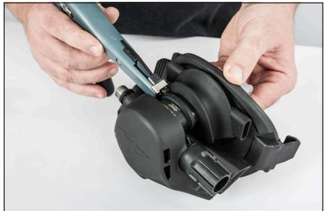
5. Fit the tie wrap P/N 520-039 into position, ensure the joint of the tie wrap ends up in the center of the side of the mouth opening as shown. Pull as tight as possible by hand or use a tie wrap installation tool. Cut
