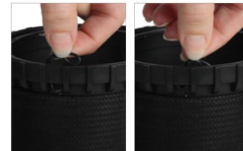
**1.4** Bend the O-ring and insert it (from the top) into the compartment next to the first. **Tip!** Use a paper clip or similar to pull/push the O-ring through the opening.
