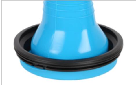
**1.7** Mount the seal onto the NEVA Ring as displayed in this image. Ensure that the flange of the seal is inserted into the groove of the NEVA Ring.
