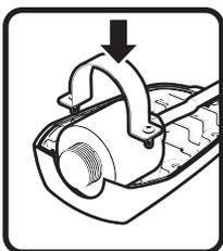
4. Remove the O2 sensor, cable, and seal into the O2 Analyzer housing.
