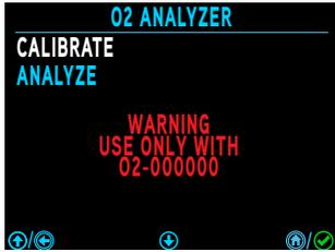
**⚠ DANGER:** Your new DSX and O<sub>2</sub> Analyzer cable are paired and precisely tuned at the factory, to compensate for resistance in the cable. **ONLY** use the cable that ships with your DSX. The cable serial number (labeled on the cable) must match the serial number that displays on your DSX (O<sub>2</sub> Analyzer Sub Menu) screen. Contact your Apeks Dealer for assistance if the Oxygen Analyzer cable ever needs to be replaced.
