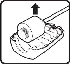
5. Carefully unplug the molex connector from the O2 sensor connector.
