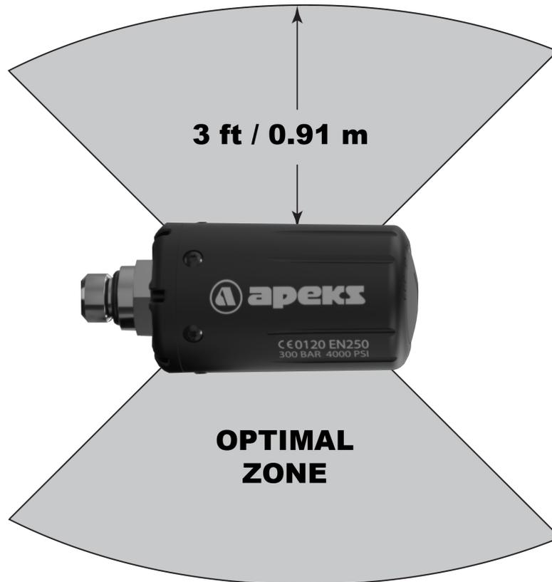
The DSX cannot effectively receive a signal when it is held out to the sides (as displayed above) of the TMT or held at distances greater than 0.91 m (3 ft) in front of the TMT. Best reception is achieved when the DSX is within less than 0.91 m (3 ft) of the TMT.
