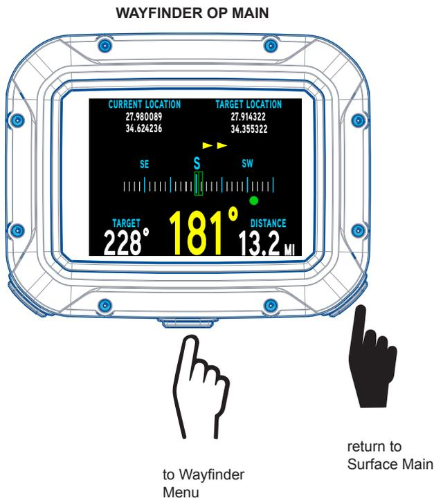
**NOTE:** The Wayfinder Op Main shall replace Compass Op Main while the Wayfinder Mode is active. When active, you may go back and forth between Surface Main and Wayfinder Op Main by holding the Right button. The Compass Op Main shall be restored again as the default function after reaching your selected target location in Wayfinder Mode or you select Exit From Wayfinder in the Wayfinder Menu.
