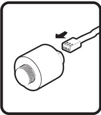
2. Place the O2 sensor, cable, and seal into the O2 Analyzer housing. Ensure the seal groove is clean and the seal is seated properly.
