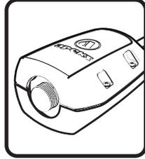
5. Screw the dome cap clockwise onto the O<sub>2</sub> sensor threads, as shown. DO NOT overtighten.
