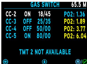
If the current PO<sub>2</sub> value is not optimal or the gas has a risk of isobaric counterdiffusion, then a warning will display when that gas is highlighted. The diver may override the DSX and force the gas switch by pressing the right button.
