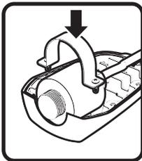
4. While ensuring not to pinch the O<sub>2</sub> analyzer cable, replace the O<sub>2</sub> analyzer housing cover. Then install the retaining screws. DO NOT overtighten.
