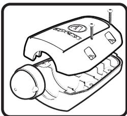
3. Remove the sensor strap, and retaining screws with a philips head screwdriver.
